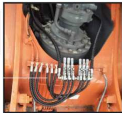
Hartex Hydraulic Grease Pump installation on EX-1200
